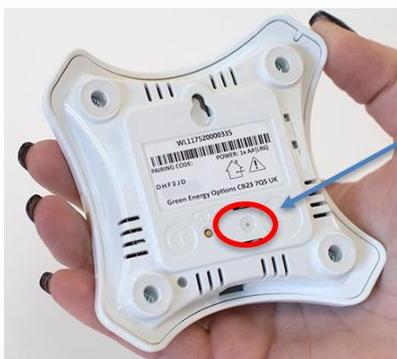
The Sensor LED is located on the underside of the device, between the 2 water detection terminals.
