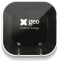
The hub is the control centre of the system in your home and communicates with each of the devices to get information or to control it. It also connects to your internet router, so it can talk to the geo cloud services and mobile applications over the Internet.
